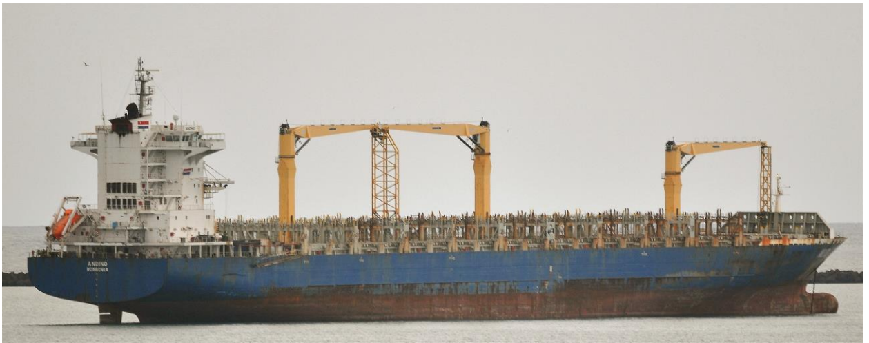
ANDINO equipped with 3x45t cranes (installed in 2016)
