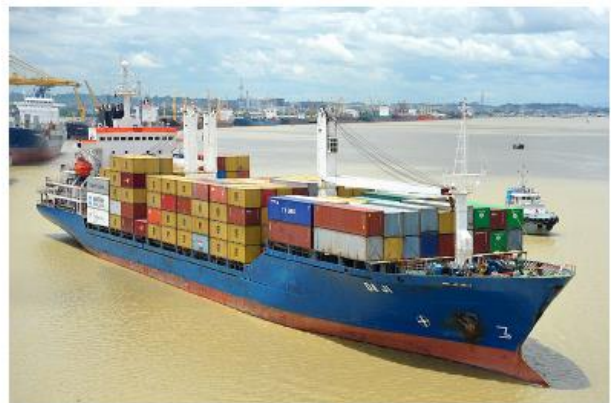
above: the 'UCC 14' vessel DA JI , originally the WATERSTOKER , upon departure from Chittagong. The type name reflected the ships' deadweight capacity of around 14,000 dwt. photo: I. Meshkov
